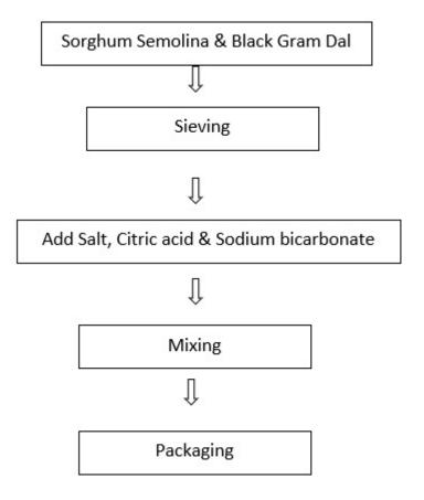
Fig 6.9 Process flow of preparing Sorghum Idli mix
