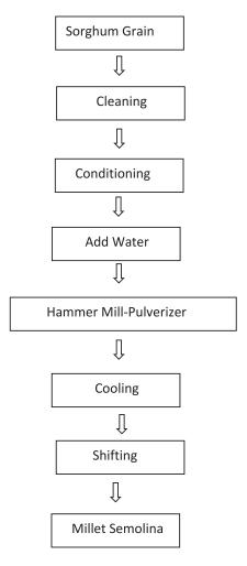
Fig 6.7 Process flow of making Millet Rava
