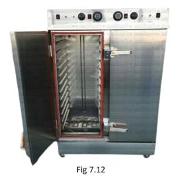
Types: Both continuous steamers and batch steamers find applications in millet-based product production. The choice depends on the production scale and desired cooking characteristics.
