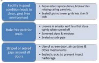
Fig. 3.8: Layout and Design factors
